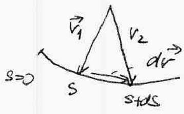
$$\text{grad } \varphi(\vec{r}) = n(\vec{r}) \cdot \vec{S}_0(\vec{r}) = n(\vec{r}) \cdot \frac{d\vec{r}}{ds} \Big|_{\vec{r}}$$
